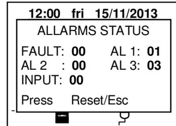
The screen can be closed by pressing the key or the key. If a new alarm occurs the screen will appear again automatically.
