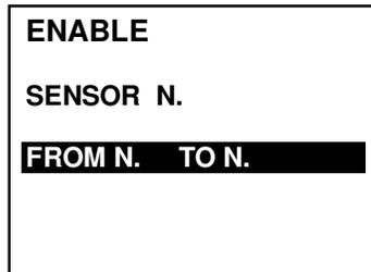
The second line, acts on a group of sensors. -----> Pressing
