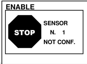
If the sensor or one of the group's sensors is not configured, a window notifies you that the operation is not possible.----->
