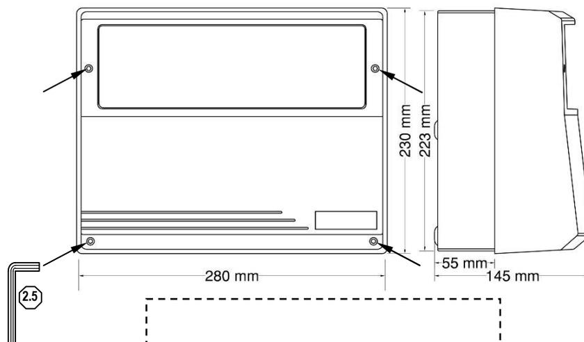
**Fig 2 – CE408P Dimensions and Template for wall mounting**
