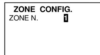
Then, use the **▲** and **▼** key, to scroll through the different items. Pressing **ENTER** on the item, the value is highlighted to indicate that it is editable. ----->
